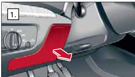
Fuse box – left-hand drive (steering wheel left)
